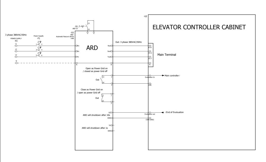
Battery: 60VDC (5x12V7AH)
